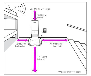
**WARNING:** To prevent the risk of your robot falling downstairs, ensure that the charging station is placed at least 4 feet (1.2 meters) away from stairs.
