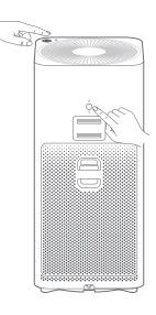
Resetting the Wi-Fi: If your phone is unable to connect to the air purifier, simultaneously press and hold the mode and the light button for 5 seconds. A beeping sound indicates that Wi-Fi has been successfully reset.
