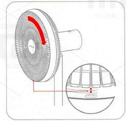
While installing the front protective mesh, turn it clockwise until two marks on lower side match.
