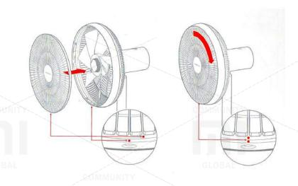
To install the front protective mesh, turn it clockwise until two marks on lower fringe match.
