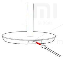
Plug a power cord into a special connector in fan base, and connect it to power supply. The corresponding beep indicates successful connection of the device to a power supply;
