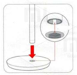
Insert the stand pole to the special socket on the device base.
