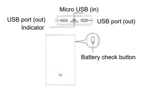
Note: the «battery check» button are not intended to turn on / off the device. This battery has the function of automatic detection of charging and discharging, so there is no need to constantly press the charge check button. In two minutes before the discharge, the amount of power LEDs are switched off.
